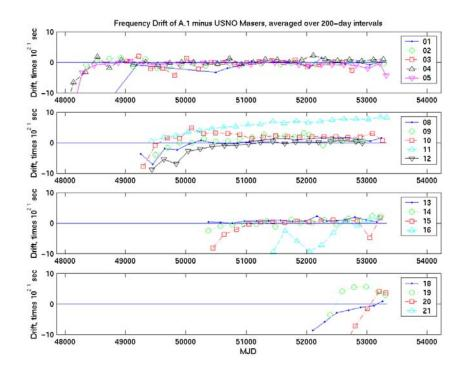
Figure 7. Frequency drifts of USNO masers located in Washington, DC (USNO-DC), computed by differencing frequencies at endpoints of 200-day intervals. Since MJD 49000, the frequency drifts between the A.1, UTC, and TT (BIPM03) have been less than  $10^{-21}$ /sec. The maser NAV21 has drifts of order 4-5  $10^{-20}$ /sec.
